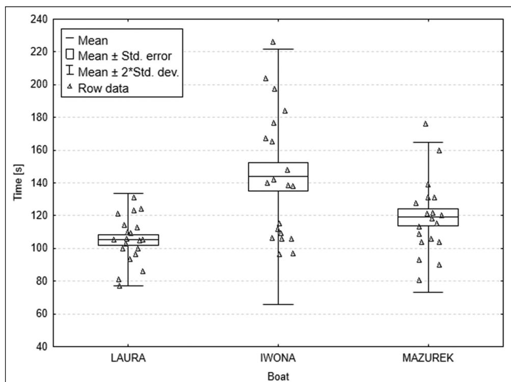
**Figure 1.** Speed of "Laura", "Iwona" and "Mazurek" rowing boats for the 100-m distance
